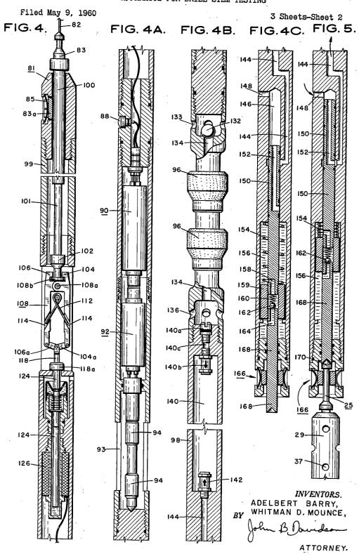
APPARATUS FOR DRILL STEM TESTING
