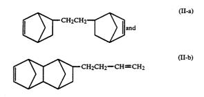
is readily metathesis polymerized or readily metathesis copolymerized with norbornene-type cycloalkene such as DCP to produce highly cross-linked heat resistant copolymers having a very high softening point.
