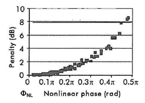
$$\phi_{NL(total)} = \sum_{span=1}^{i} \frac{2\pi}{\lambda} \left( \frac{n_2 P_i L_{eff}}{A_{eff}} \Big|_{Line} + \frac{n_2 P_i L_{eff}}{A_{eff}} \Big|_{DCF} \right)$$
