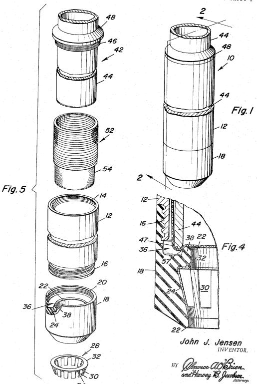
CORE BARREL INNER TUBE
