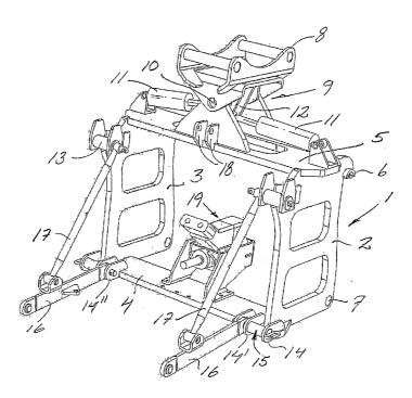
(57) Abstract: The invention relates to a tool holder arranged, on one hand, to be coupled to a working vehicle and, on the other hand, to be coupled to a tool, comprising vehicle- coupling members for alternative coupling to different working vehicles as well as tool-coupling members for alternative coupling to different types of working tools. The tool holder is particularly characterized by a driving member carried on the tool holder and intended to drive a coupled tool.
