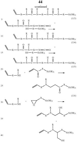
The alkenylsilane compounds (j) include compounds having a silicon-containing functional group, a polar component part and an alkenyl group in the molecule. Such compounds are available as commercial products. Examples of the commercial products include, but are not limited to, products manufactured by Shin-Etsu Chemical (trade name: KBM576, X-12-575, X-12-577, X-12-563B and X-12-565) and the like.
