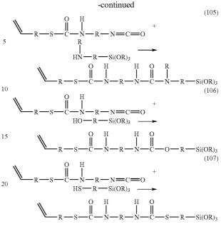
The reaction product (j-8) in the reaction of the mercapto group of a thiol compound represented by general formula (84) above with the  $\alpha$ , $\beta$ -unsaturated carbonyl group of compound (i) can be prepared according to the reaction method (1) described above. At this time, the reaction represented by the following general formula (108) progresses.
