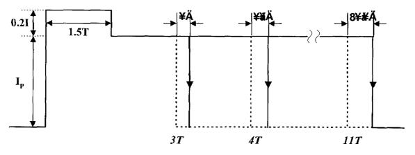
Dotted Line : Write Strategy specified for a disk Solid Line : Write Strategy adjusted based on track pitch difference
