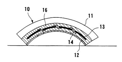
(57) Abstract: A semiconductor crystal substrate (13) is fixed in a bent state to a support body. Preferably, the semiconductor crystal substrate (13) is bonded to a transparent resin member (16) provided between a surface cover member (11) and a back cover member (12).
