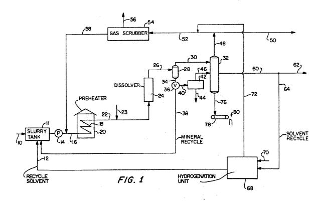
Coal liquefaction process employing octahydrophenanthrene-enriched solvent.
