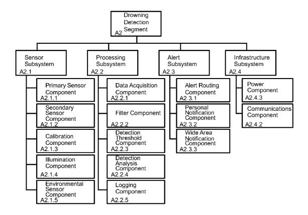
**Figure 3. Drowning Detection Architecture**
