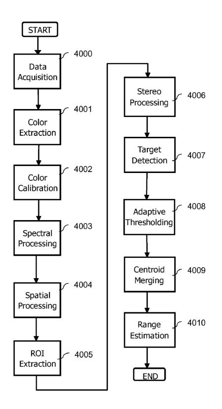
Figure 4. Drowning detection processing
