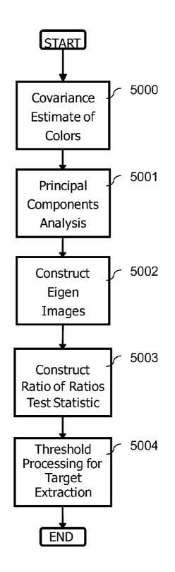
Figure 5. Processing steps for performing spectral processing
