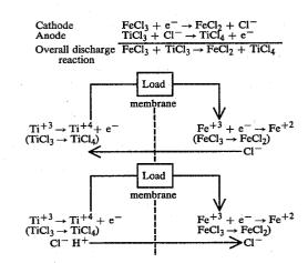
The ion transport material is used in an amount of from about 50 to 20 volume % as compared with about 50 to 80 volume % of the rubber. Preferably, the amount of the ion transport material is about 30 to 35 volume %. Utilization of more than about 50 volume % of the ion transport material may result in the creation of holes greater than 100 angstroms which can cause intermixing of the two couple solutions resulting in a lower effeciency of the redox cell.
