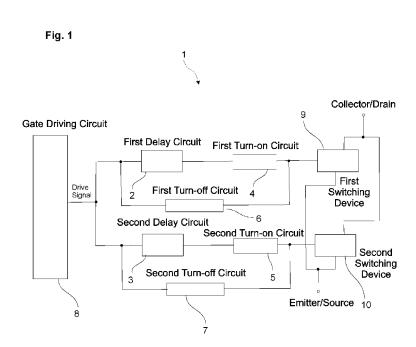
(57) Abstract: The present invention relates to a power electrical switching circuit and more particularly to parallel-coupled switching devices and an associated switched-mode power converter (1). The present invention more particularly relates to a switched-mode power converter (1) comprising a first switching device (9) connected electrically in parallel to a second switching device (9), the first and second switching devices (9 and 10) being driven by a gate driving circuit (8).
