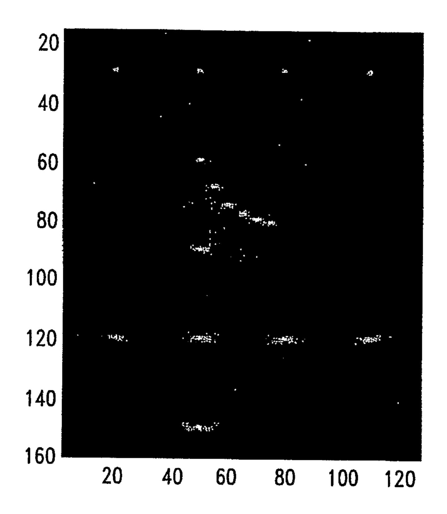
SPATIALLY COMPOUNDED IMAGE RECONSTRUCTION USING UNIFORM ILLUMINATION METHOD. FIVE FLAT WAVEFRONT PULSES WERE USED AT STEERING ANGLES OF -20, -10, 0, 10, AND 20 DEGREES. INTENSITY DATA ARE COMPRESSED WITH A SQUARE ROOT FUNCTION.
