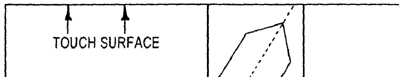
NON-PERPENDICULAR POINTER APPROACHING TOUCH SURFACE CALCULATED CENTER LINE SHOWS EXPECTED POINT OF CONTACT.
