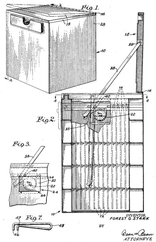
VERTICAL FILING CABINET COVER AND CONTROL MECHANISM THEREOF
