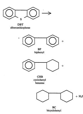
The hydrodesulfurization activity or zero order rate constant, k, for the catalyst was found to be  $15 \times 10^{16}$  55 molecules of DBT desulfurized per gram of catalyst per second. This activity was determined at a DBT conversion level  $\leq 50\%$ . The results are summarized in Table I.
