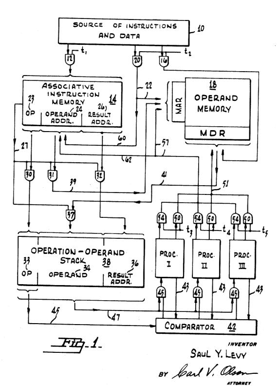
Sept. 30, 1969 S. Y. LEVY 3,470,540 MULTIPROCESSING COMPUTER SYSTEM WITH SPECIAL INSTRUCTION SEQUENCING Filed April 24, 1967 2 Sheets-Sheet 2
