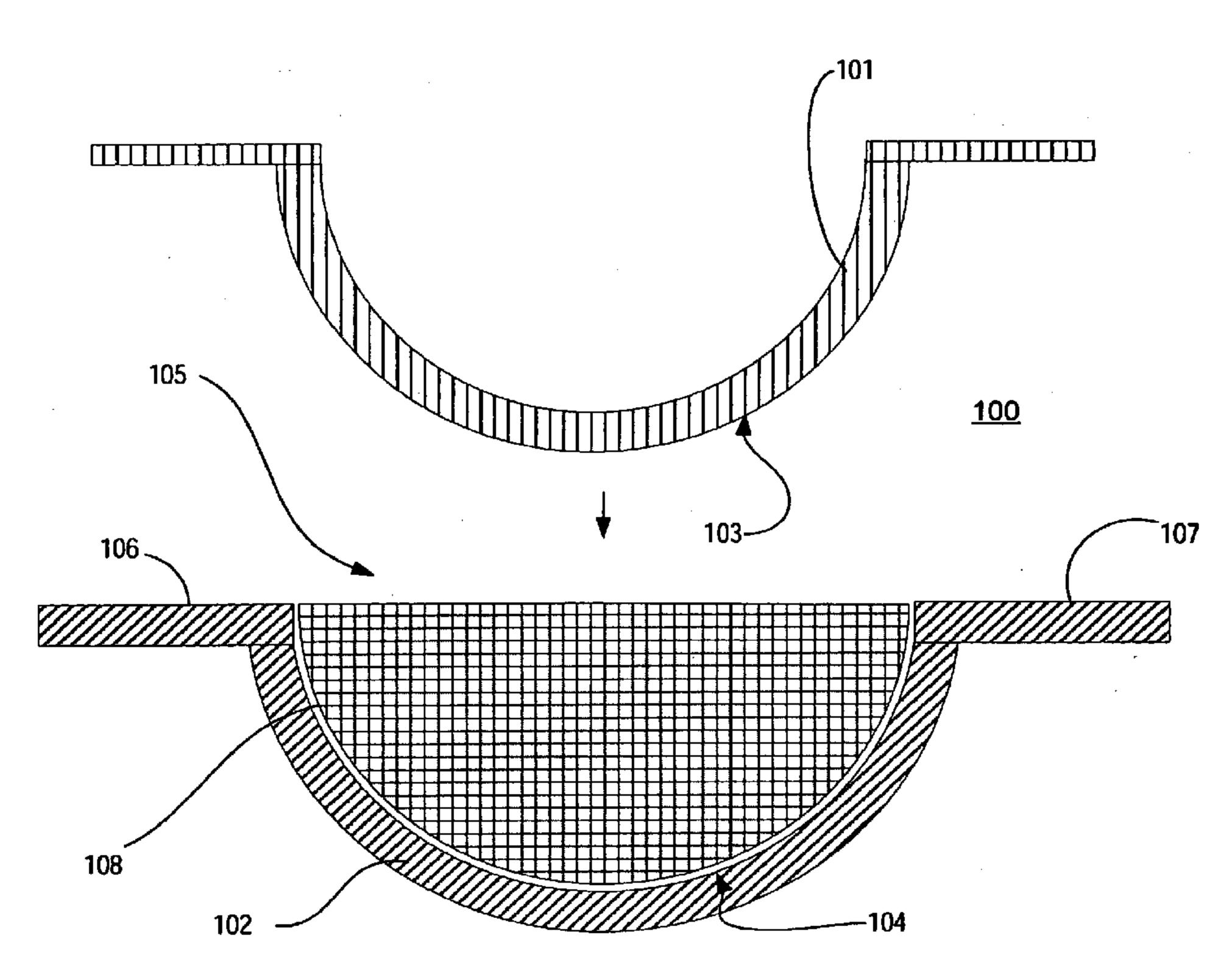
(57) Abstract: The present invention includes methods and appartus for the reduction of excess polymeric flash ring during forming of an ophthalmic lens, in a area defined by a first mold part (102) and a second mold part (101) wherein during the formation of the ophthalmic lense a HEMA is formed and the HEMA ring and a greater adhesive force is generated on the HEMA ring by the second mold part than the first mold part.
