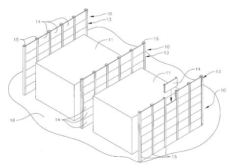
(57) Abstract: A highly protective firewall (13) supported between upstanding columns or beams (15). The firewall is made of an inorganic cementitious material which is preferably inorganic phosphate cement. In one form, the firewall comprises a group of vertically stacked panels (14) made of such material, and the panels are in turn formed by a plurality of elongated and vertically stacked hollow members (21) of the same material.
