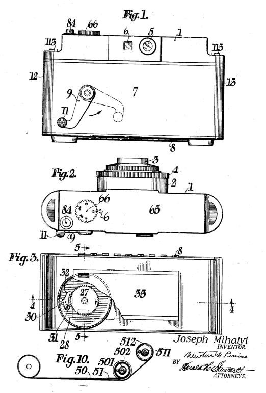
CAMERA SHUTTER SETTING AND FILM WINDING MECHANISM
