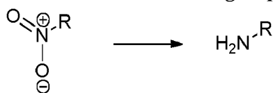
Scheme 18. Reduction of a nitro group to an amine using Fe (General Procedure R)
