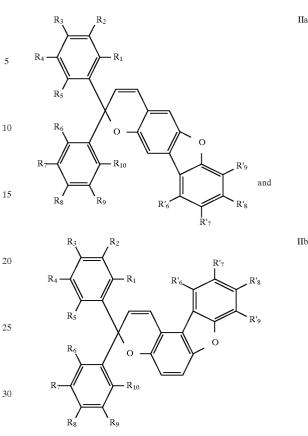
The method set forth later in this application for producing the photochromic benzopyran compounds of graphic formulas IIa and IIb forms a photochromic reaction product that includes two benzopyran compounds, namely, a structural isomer that meets graphic formula IIa and another structural isomer meeting graphic formula IIb,
