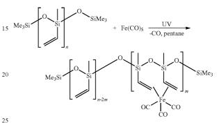
In the Schlenck's tube (Pyrex glass) equipped with magnetic stirrer condenser with oil valve 2.00 g of polyvinylsiloxane (homo-polymer), 0.363 (1.85 mmol) Fe(CO)<sub>5</sub> and 20 mL of pentane were placed. After filtration by a cannula system the mixture obtained was irradiated with UV light for 2 hours then the solvent was evaporated from yellow solution and yellow oil was dried under vacuum.
