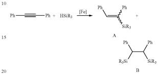
where [Fe] represents the concentration of one of the iron complex catalysts prepared above in Examples 1 to 12.
