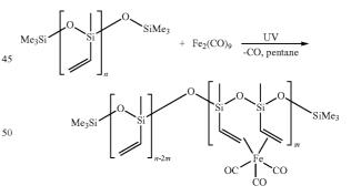
In the Schlenck's tube (Pyrex glass) equipped with magnetic stirrer, condenser with oil valve 2.00 g of polyvinylsiloxane (homo-polymer) 0.35 g (0.962 mmol) Fe<sub>2</sub>(CO)<sub>9</sub> and 10 mL of pentane were placed. The mixture obtained was stirred over-night and then irradiated with UV light for 2
