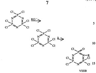
Both phosphazane VIIIA and VIIIB can thermally cleave to zwitterions (IX) to effect the initiator species 20 similar to that accepted as the initiator species in the uncatalyzed thermal polymerization of  $(NPCl_2)_{\nu}$  raw materials.
