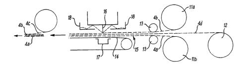
(57) Abstract: Leather sheet material is made by hydroentangling a web (4) of mixed reclaimed leather fibres and synthetic fibres. The synthetic fibres are meltable bicomponent fibres which are heated prior to entanglement to fuse and form a supporting network for the leather fibres. A sheet of tissue paper (1a) is laid over the surface of the leather fibre web (4) and hydroentanglement jets (16) are directed through the tissue paper into the web.
