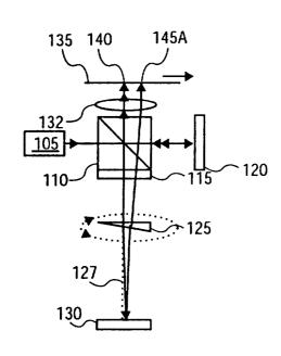
(57) Abstract: A rotatable optical wedge (125) disposed relative to a reflective member (130) and rotated between a first position and a second position to direct a light beam (127) reflected from the reflective member (130) to a position on a recording medium (135) and the position of the light beam is adjusted by moving the optical wedge (125) to different positions including the first and second positions.
