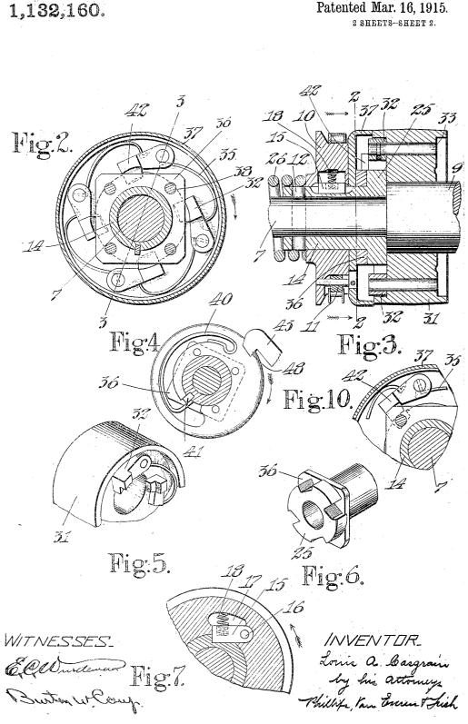
L. A. CASGRAIN. STARTING DEVICE FOR INTERNAL COMBUSTION MOTORS. APPLICATION FILED JUNE 26, 1912.
