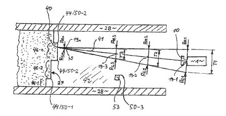
placed in relationship with an area that is released to be traveled on by the autonomous vehicle, with the result that the navigability of the travel path of the autonomous vehicle is checked, and in the case of detected non-navigability the travel path is adapted autonomously to the requirements of the situational spatial surroundings and is replaced by an alternative travel path.
