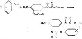
wherein R stands for any substituent(s) on the phenol which will result in the high molecular weight, nonvolatile substituted phenol which is suitable for use as the blocking agent of this invention.
