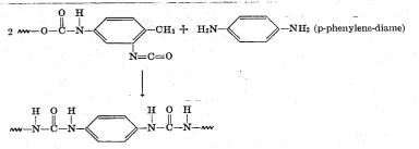
The general reaction for the cure of a blocked urethane prepolymer with a diamine is the same as above except for the additional release of two molecules of the blocking agent per molecule of the diamine. 40
