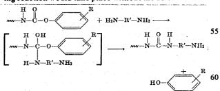
This reaction is affected by the basicity of the amine; i.e., if the amine is a strong base and rich in electrons, then the reaction is very difficult to completely prevent even with the stabilizing acid present. 65
