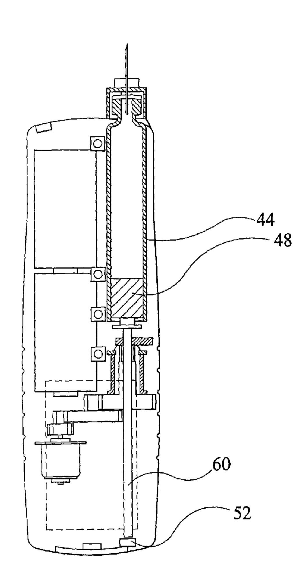
(57) Abstract: An injection device for injection of a medicament from a medicament cartridge 40 is disclosed. The injection device comprises a main housing 4, a piston 50 and an end stop switch 52 in which access to the main body 4 for replacement of the medicament cartridge 40 may only be obtained when the piston 50 trips the end stop switch.
