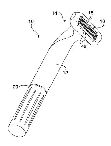
(57) Abstract: A shaving apparatus includes a reservoir (23) for storing a shaving aid material, a razor cartridge (16) having at least one razor blade (18), and a valve (26, 126) selectively actuatable by movement of the razor cartridge between a first position and a second position. In the first position the valve permits passage of a shaving aid material from the reservoir, and in the second position the valve substantially prevents the passage of the shaving aid material from the reservoir.
