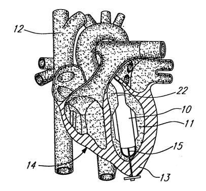
motor drive comprises a set of windings enclosed in the stationary housing structure, and a set of elongated axial permanent magnets embedded in the shroud. The axial flow blood pump can be used in an implantable ventricular assist device. The enclosed-impeller axial flow geometry of the pump, as well as the small diameter of the central hub substantially increase the volume of blood the pump is capable of containing and therefore of pumping.
