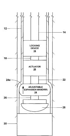
(57) **Abstract:** An apparatus (10) and method for forming a mono diameter wellbore casing (12).
