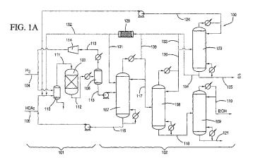
(57) **Abstract**: Recovery of ethanol from a crude ethanol product obtained from the hydrogenation of acetic acid by hydrolyzing a portion of the crude ethanol product or one or more derivative streams obtained therefrom. The one or more derivative streams comprise ethyl acetate and the hydrolyzed stream is directly or indirectly fed to the distillation zone or the hydrogenation reactor.
