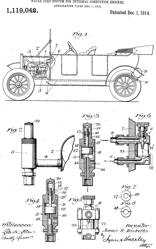
J. R. RICKETTS. WATER FEED SYSTEM FOR INTERNAL COMBUSTION ENGINES.
