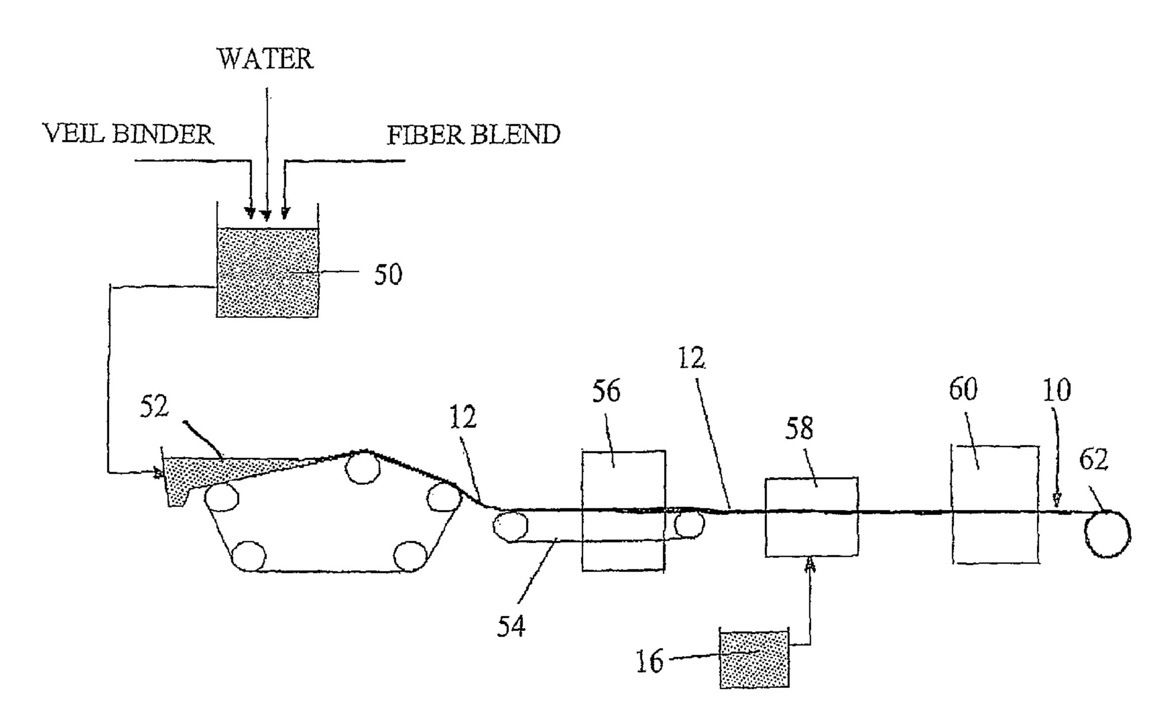
(57) Abstract: A precursor of a fiber reinforced foam structure includes a base veil having between about 50 and about 75 weight percent reinforcement fibers and between about 50 and about 25 weight percent veil binder. The base veil has a weight per unit area of between about 35 and about 400 g/m2. Further the base veil is impregnated with an expandable binder in an amount of between about 20 to about 200 g/m2.
