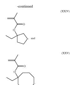
**[0030]** The photoresist compositions of the invention are not limited to any specific form of the second repeating unit. The polymer of the invention preferably includes about 20-60 mole % of the second repeating unit, more preferably about 30-50 mole %.
