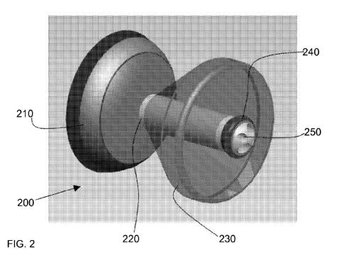
(57) Abstract: At least one exemplary embodiment is directed toward an earpiece with a sealing section for acoustically sealing the meatus of a human ear, which includes an inner ear canal speaker; an inner ear canal microphone; connected to a logic circuit which can include a digital signal processor (DSP), where the sealing section touches a portion of the ear canal to substantially acoustically seal the meatus of a human ear canal.
