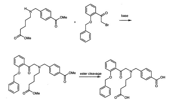
5 If (VI) represents, for example, methyl 5-{[2-(benzyloxy)phenethyl]amino}pentanoate and (VII) represents methyl 4-(bromomethyl)-benzoate, processes C and E can be represented as shown in the scheme below:
