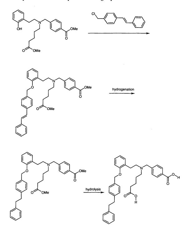
Example of the reaction sequence according to processes D/G/E
