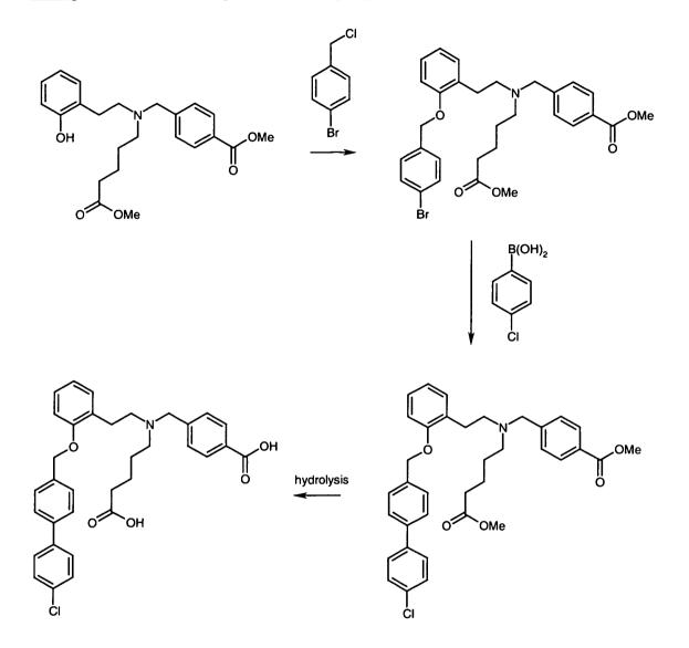
Example of the reaction sequence according to processes D/F/E
