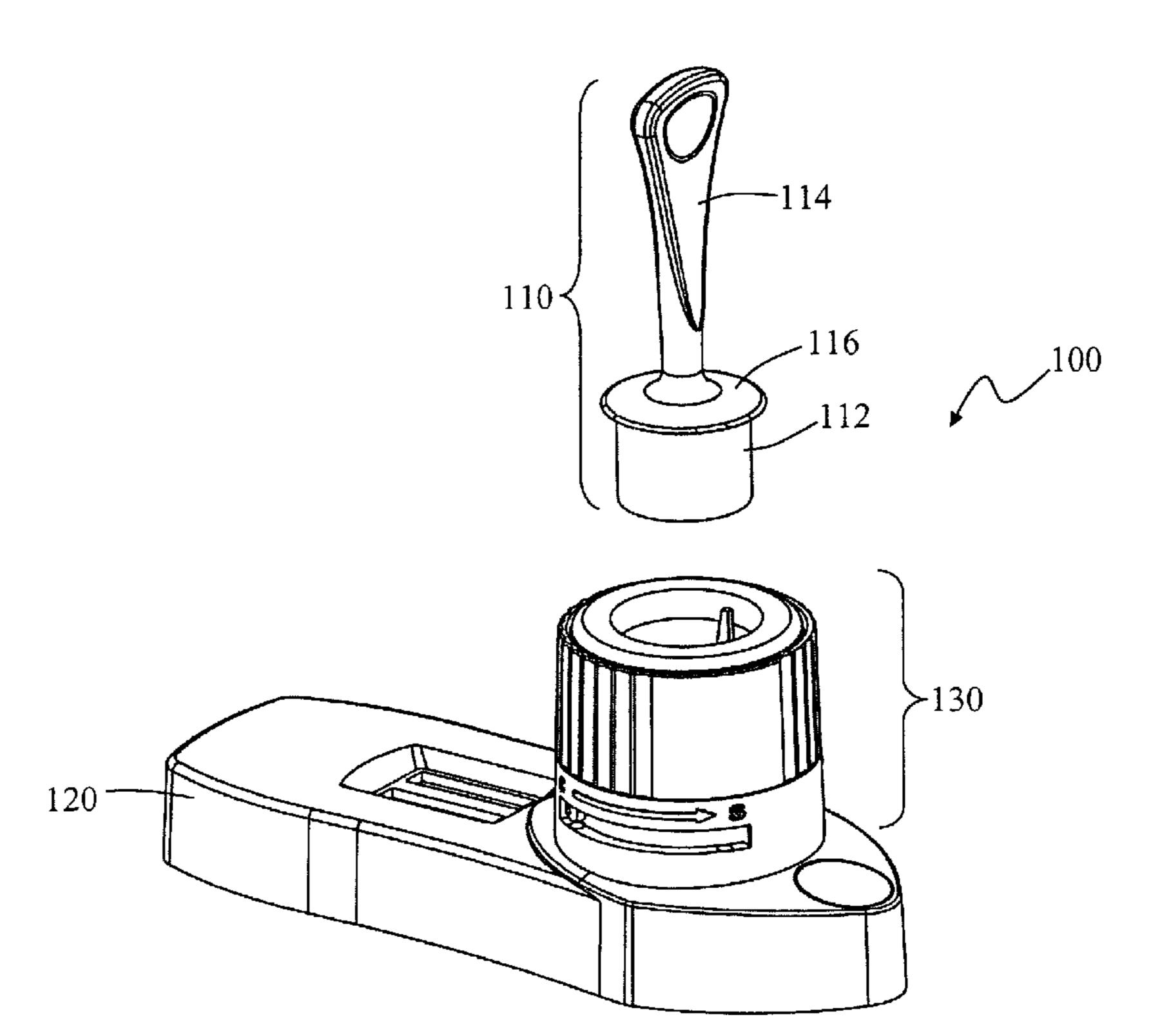
(57) Abstract: A device (100) comprising a casing (120), a sample collection well (130) and a sample applicator (110). The sample applicator (110) further comprises a rigid handle (114), a rime (116) and an absorbent member (112).
