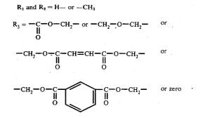
These include: glycidyl acrylate, glycidyl methacrylate, allyl glycidyl ether, methallyl glycidyl ether, glycidyl crotonate, vinyl glycidyl ether, allyl glycidyl maleate, allyl glycidyl phthalate and butadiene monoxide. 35
