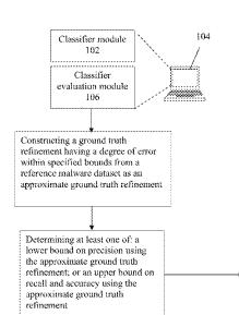
Evaluating a classifier for at least one task of a classification method or a clustering method by examining changes to the at least of one of the upper bound or the lower bound produced by the approximate ground truth refinement
