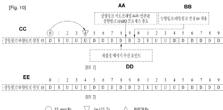
AA ... Terminate uplink HARQ process associated with uplink subframe #4
