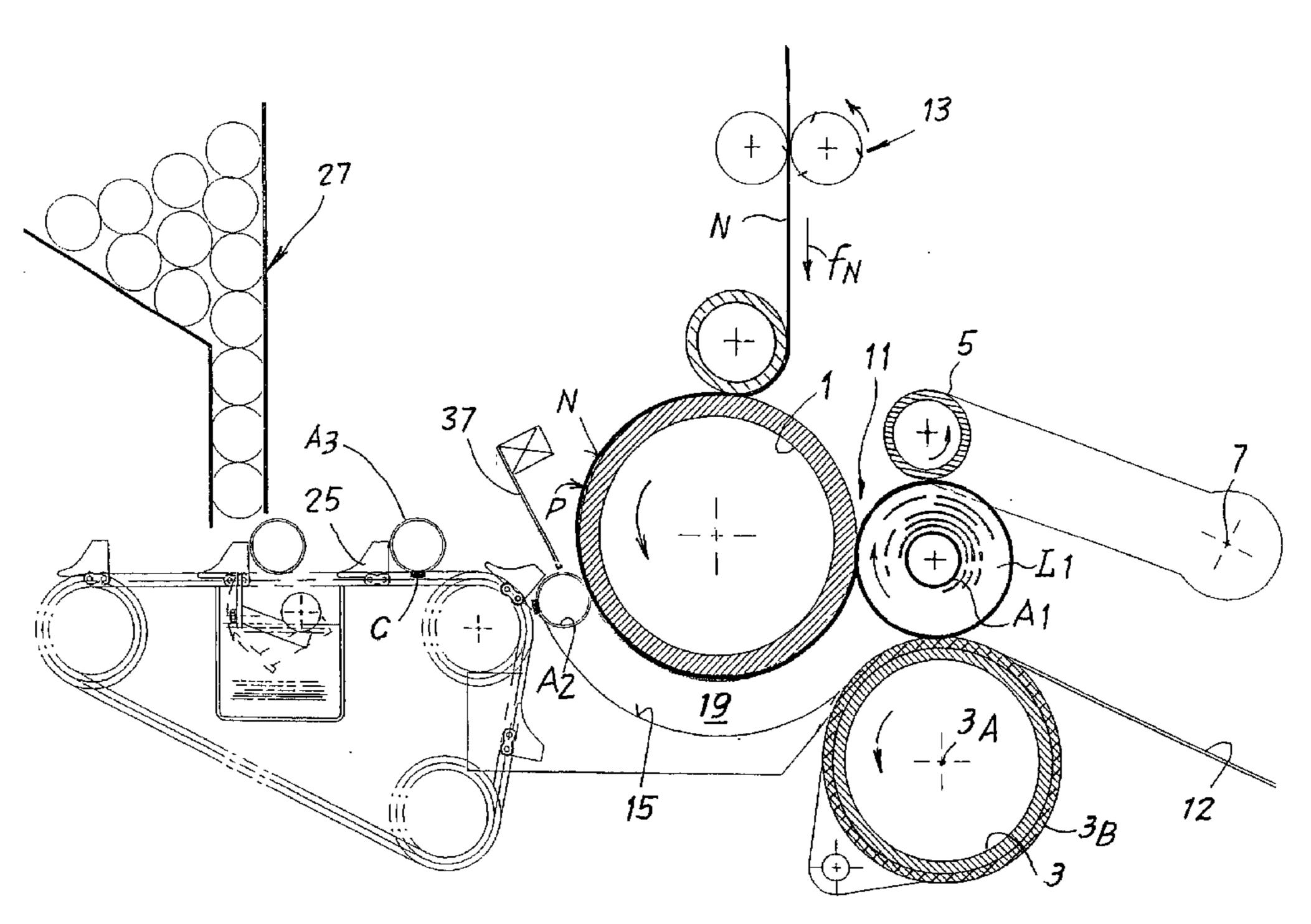
(57) Abstract: A method for producing logs (L1, L2) of web material (N) wound around tubular cores wherein the tubular core (A1-A4) is equipped with glue to secure the initial end of the web material and allow winding. Part of the glue applied to the tubular core is transferred to the web material (N) before it is severed upon termination of winding the log, to seal the final free end of the formed log.
