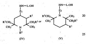
The aminoalcohol IV can be prepared by hydroxyalkylation of the corresponding primary amine. Another method is the reductive amination of the 4-oxo- 30 piperidine with the appropriate aminoalcohol. Some classes of polyalkylated 4-aminopiperidine derivatives are disclosed in U.S. Pat. Nos. 3,684,765, 3,904,581 and 4,166,813.
