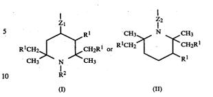
in which R<sup>1</sup> is hydrogen or alkyl having 1 to 4 carbon atoms, R<sup>2</sup> is hydrogen, alkyl having 1 to 12 carbon atoms, allyl, benzyl, acetyl, acryloyl or cyano, Z<sub>1</sub> is a direct bond, --NHCH<sub>2</sub>CH<sub>2</sub>--, --NHCH<sub>2</sub>CH<sub>2</sub>CH<sub>2</sub>-or --OCH<sub>2</sub>CH<sub>2</sub>--, with the heteroatom attached to the piperidyl ring, Z<sub>2</sub> is ethylene or trimethylene,
