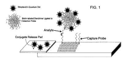
(57) Abstract: The invention provides semiconductor nanocrystal-based lateral flow microarrays (SN-LFM), assays using SN-LFM, signal amplification strategies, optical detection devices for collecting data from SN-LFM assays, and integrated sample-toanswer SN-LFM assay/detection devices.
