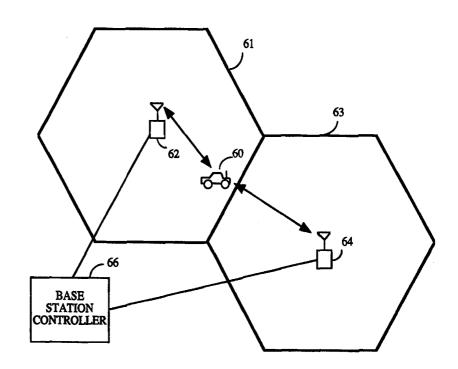
mobile station. A series of computations described in detail herein are performed upon the measured time values to determine the time difference between the slave base station (64) and an adjustment of the slave base station (64) timing is performed in accordance therewith.
