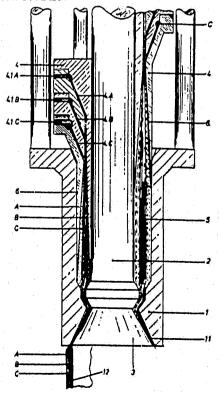
Method and Apparatus for the Discontinuous Manufacture of Co-Extruded, Hose-Like Multi-Layer Preforms from Thermoplastic Material to Form Large-Volume Multi-Layer Hollow Bodies
