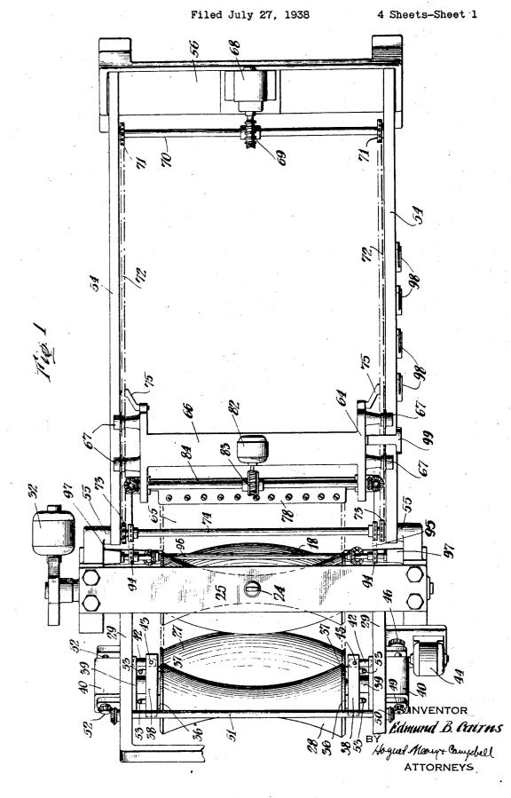
METHOD AND APPARATUS FOR ROLLING CURVED SHEETS
