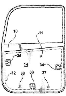
(57) Abstract: A barrier panel (1) for vehicle door assemblies that is provided with snap attachment structures (3, 15) that extend outward from an outboard side thereof . The snap attachment structures (3, 15) are configured to engage various structures, including notches, tabs and/or individual discrete holes provided in the inboard surface of a door panel (2, 10).
